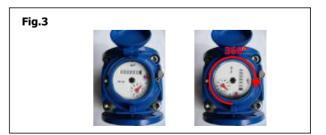
The meter totalizer must be legible and accessible for any maintenance operations. For this purpose, the screen can rotate 360° around its axis (before sealing the cover), facilitating the reading of the totalized volumes (Fig.3).
